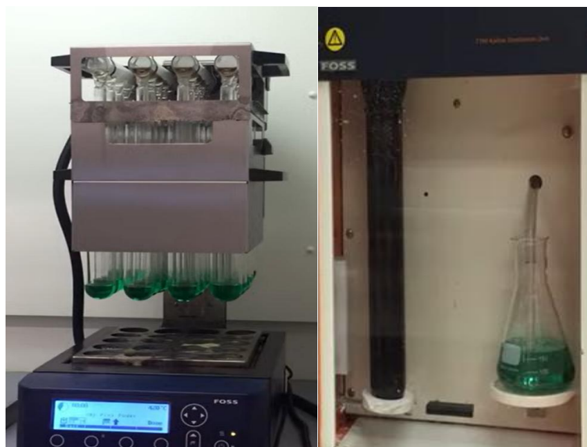
Figure 18. Kjeldahl Method for Determining Nitrogen Content
