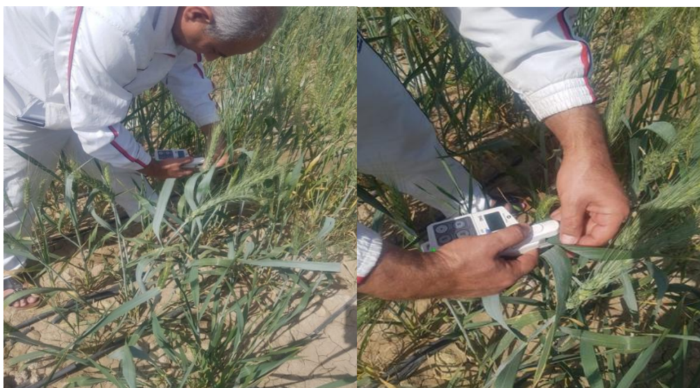
Figure 16. Measurement of chlorophyll content using SPAD.
