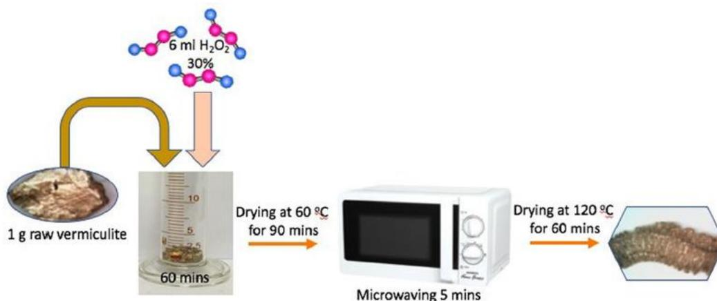
**Figure 14** Schematic of the modified vermiculite preparation process
