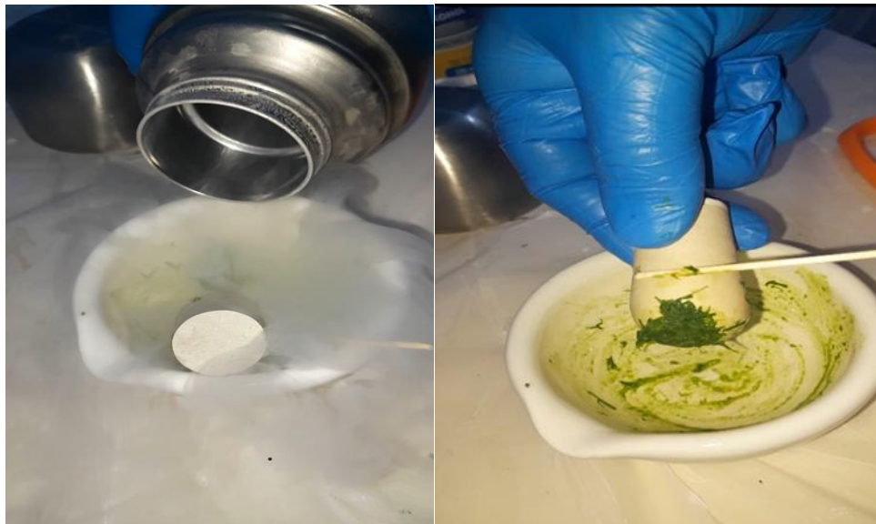
Figure 22. Crush the walls using liquid nitrogen.
