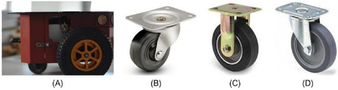
Figure 1.4. Conventional wheels (A) fixed wheel, (B) caster wheel, (C) powered steering wheel without any offset, and (D) powered steering wheel with longitudinal offset [44]
