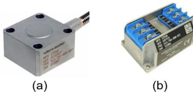
Figure 3. Equipment used to measure the vibration velocity of turbines in Kirkuk Gas power plant, (a) The CA 202 accelerometer, (b) the signal conditioner IPC 704 converts a charge-based signal from a piezoelectric transducer into a current or voltage signal.
