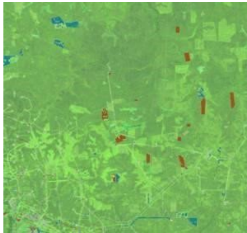
Figure 5 - Fragment of a color-synthesized image with the classification of appeared and disappeared objects
